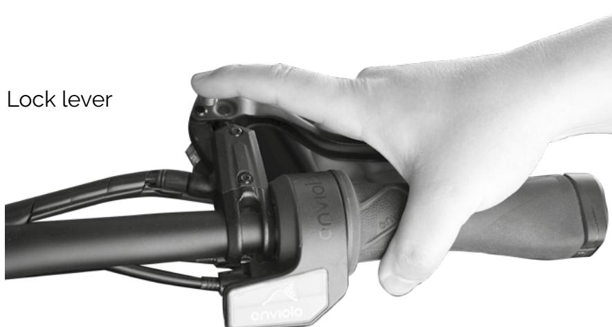
The parking brake should only be used when loading goods or children onto the cargo bike. The parking brake on the front wheels is activated/deactivated with the small lock lever.
