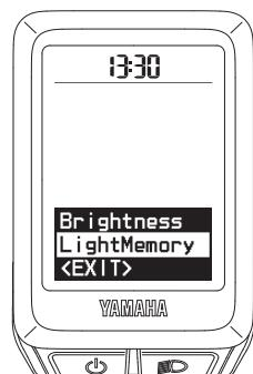
Sets whether to ignore or save the on or off status of the headlight when the power of the e-Bike Systems is turned off.
