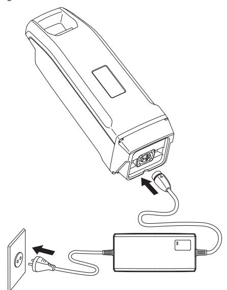
6. See "Reading the charging status for Battery Pack", and check that the Battery Charger is charging the Battery Pack.
