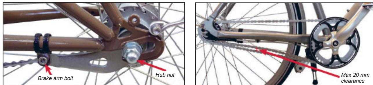
To adjust the chain, loosen the hub nuts and the bolt in the rear hub brake arm. Then move the rear wheel forward or backward so that the chain gets the desired clearance. Remember to tighten the hub nuts and the brake arm bolt and check that the wheel sits right in the middle of the rear fork.
