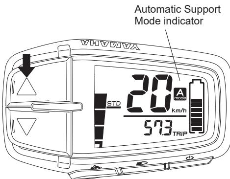
The Automatic Support Mode, which enables automatic change to the optimal assist mode according to the riding conditions, can also be used.
