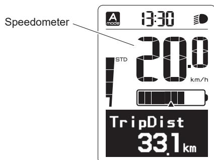
The speedometer displays your bicycle speed (in kilometer per hour or mile per hour). To select the km/mile, see "Settings".
