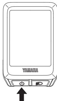
Each time you press the power switch, the power is turned on and off.
