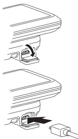
Power can be supplied to most external devices (e.g. various smart phones etc.) by connecting a commercial USB 2.0 OTG cable.
