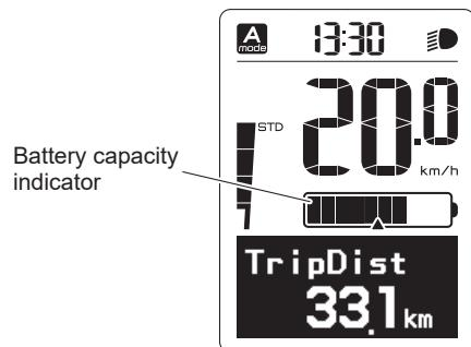
The battery capacity indicator displays an estimate of how much capacity is left in the Battery Pack.
