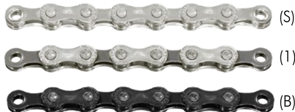
CN10A [1/2" x 11/128"] [Chromized Pins] [Chromoly Plates] S[Silver] / 1[Silver/Gray] / B[Black] 266g [110L]
