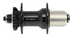
HBMX92 [142mm x12mm] X90 [135mm x10mm] [A7075 Alloy Cassette Carrier] [Sealed Cartridge Bearings] [Only for CSMZX1/Z91/X9 Cassette] 310g[w/o QR]
