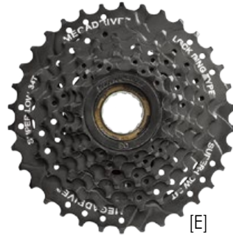
MFM300 7CV 13-34T 7DV 14-34T [7-Speed] [Lockring Design] E[ED Black] 2[Brown+ED Black]
