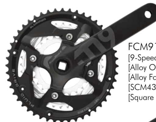
FCM950 40-30-22T [9-Speed] [Alloy Outer Chainring] [Alloy Forged Cranks] [SCM435 Bolts & Nuts] [Chromoly Axle] 1071g[incl. BB]
