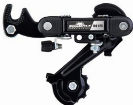
RDM15 LD/LB SD/SB [5-Speed] [14-28T] [Indexed Adjuster]
