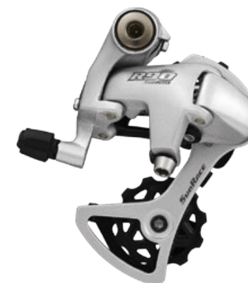
RDR91 SD/LD [9-Speed] [11-28T] [Alloy Bracket & Outer Link] 257g[SD] / 279g[LD]
