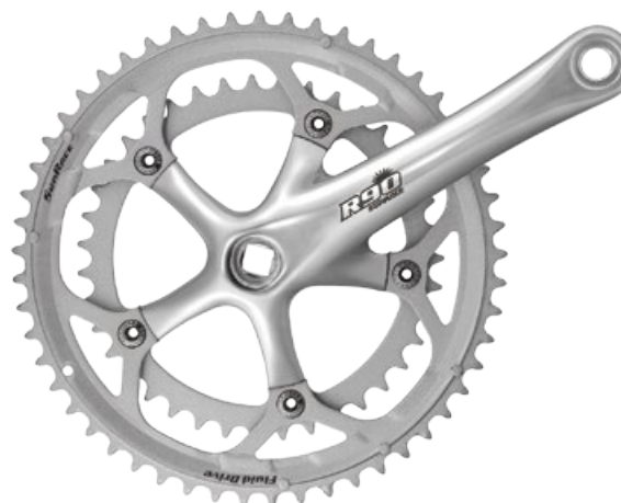
FCR96 50-34T FCR910 53-39T [9-Speed] [SCM435 Bolts & Nuts] [6061 Forged Alloy Crank] 831g[96] / 889g[91]
