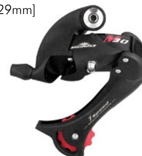
RDM37 LD/LB/SD/SB [7-Speed] [13-30T] [Indexed Adjuster]
